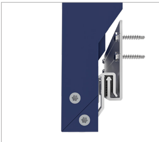
Position of the Z- and S-brackets on the shaped cassette.
