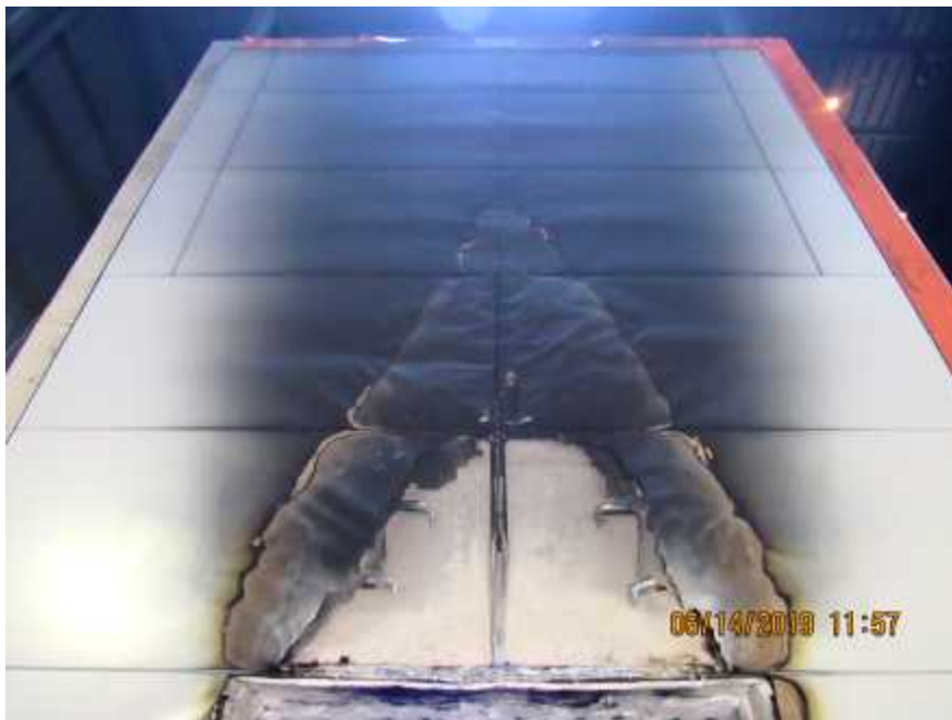
Photo No. 16 Post Test View of Panels
