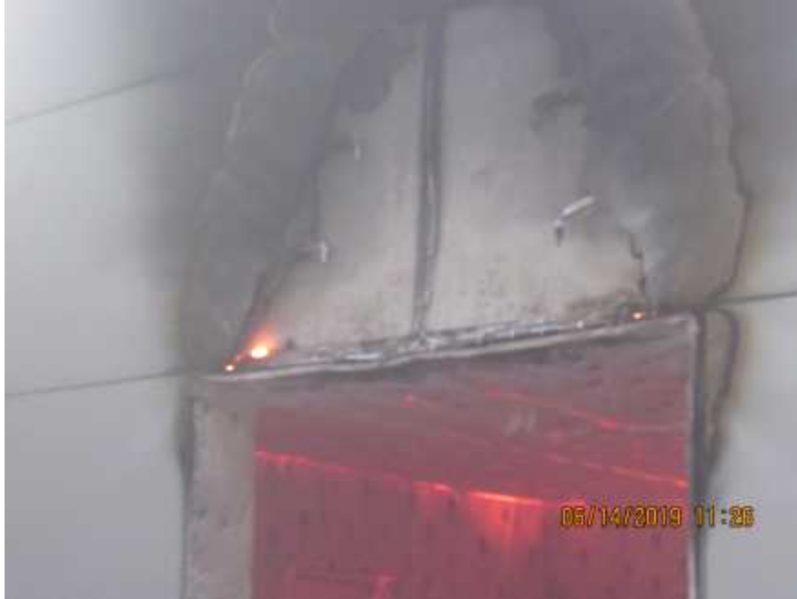
Photo No. 15 Sustained Flaming After End of Test
