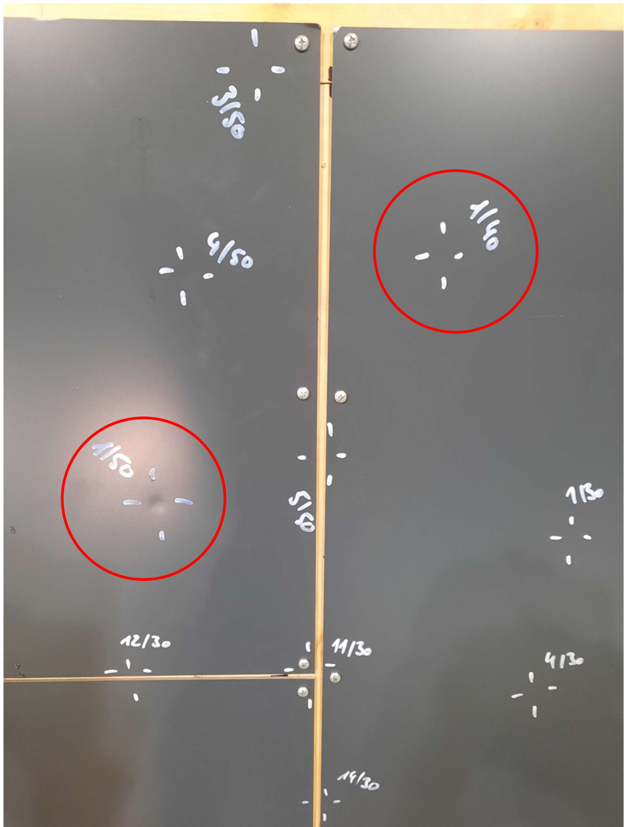
Pic. 3 Visible dents after shooting with 5 cm IB (1/50) and 4 cm IB (1/40)
