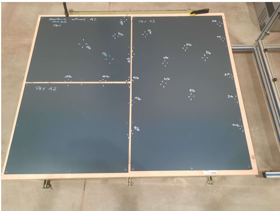
Pic. 2 Test specimen 1 overview of shooting points
