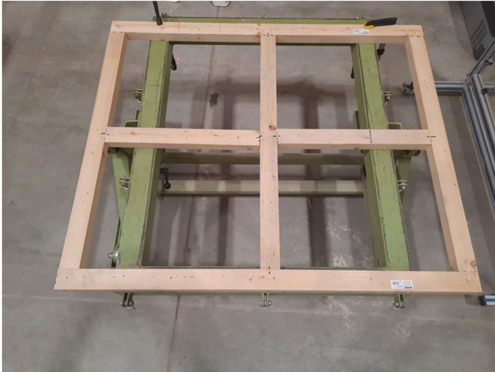
Pic. 1 Substructure Wooden bar 60/40 mm
